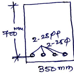
$$f_{ck} = 20 \text{ N/mm}^2 \quad f_y = 415 \text{ N/mm}^2 \quad A_{st} = 2213.5 \text{ mm}^2$$
