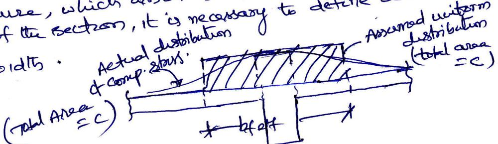
③ @ when the dimensions of the beam is fixed, and when the actual UBM due to loads exceeds the limiting Moment of resistance of a SRS, the strength of the section can be increased by providing reinforcement in Comp Zone in addition to the reinforcement in tension zone. If the section is provided with both tension and comp. reinforcements then the section is called "DRS".
