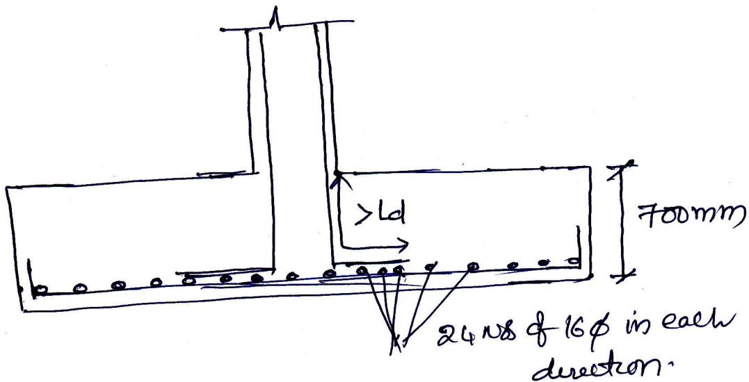
Transfer of force at the base should be checked
